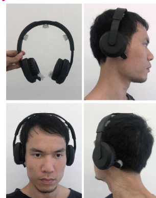
Compact, Wireless, and Quick-to-Apply EEG Sensor
