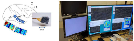
Visualization of functional maps with spatial resolution at electrode spacing (400μm)
